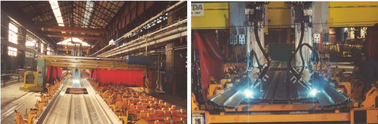
Fig. 9: Tandem welding in rail vehicle construction. Welding speed achieved: 250 cm / min.
